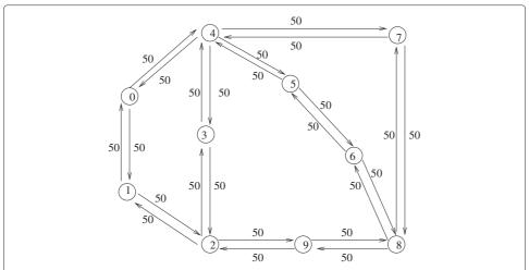
**Figure 2 Test network**  $\mathcal{E}$ **.** This test network (with the indication of the bandwidth of each arc  $C'_{k'}$  in Mbps) is in [25].
