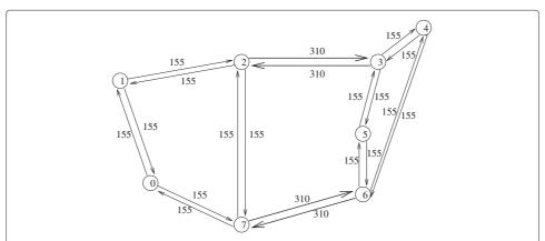
**Figure 1 Test network**  $\mathcal{M}$ . This test network (with the indication of the bandwidth of each arc  $C'_{k'}$  in Mbps) is in [24].
